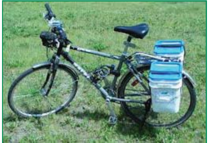
Rain Proof Bucket Panniers. Directions to make your own: http://tinyurl.com/bucketpanniers
